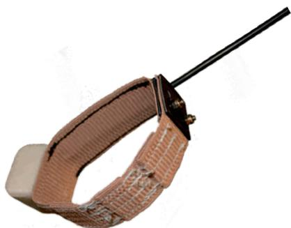
The Expandable Fawn Collar has been designed for attaching a UHF-ID tag on a fawn. This collar is very light and made of elastic material which is folded in several layers. The layers are sewed together with cotton yarns, which allow the layers to unfold with the effect from wear, time and weather. The combination of elastic and folded material ensures a good fit for a growing neck of the fawn.
