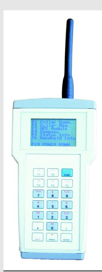
The GPS Plus Handheld Terminal provides the wireless radio interface between a PC and the GPS-Plus collar.
