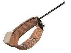
The Expandable Fawn Collar has been designed for attaching a UHF-ID tag on a fawn. This collar is very light and made of elastic material which is folded in several layers. The layers are sewed together with cotton yarns, which allow the layers to unfold with the effect from wear, time and weather. The combination of elastic and folded material ensures a good fit for a growing neck of the fawn.
