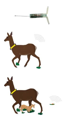
To locate the calving site, the VIT is equipped with a VHF beacon transmitter. Before implanting the VIT, it is possible to program the VHF beacon to transmit only on certain days and hours. The VHF beacon pulse rate will double when the VIT is pushed out of the mothers body.
