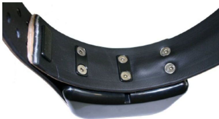
Figure 60: Attachment of curved battery pack to round collar with two metal base plates (left) and two Fastlock washers (right)
