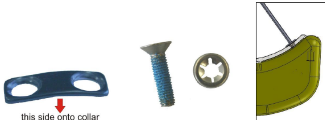
Figure 61: Attachment for curved battery pack on round collar. Left: metal base plate; centre: screw and Fastlock washer; right: angle to attach screws
